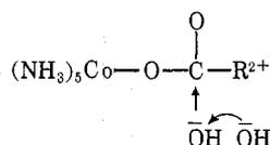
In the case of the trifluoroacetato complex the low activation energy for this path (6.8 kcal mole<sup>-1</sup>) only seems consistent with a concerted mechanism with considerable bond making in the activated complex. The results on the chloroacetato complexes presented here could be interpreted on the basis of the same mechanism. However, the activation energies for the latter complex do not require a concerted mechanism, and an intermediate (I) may form by reaction with one
